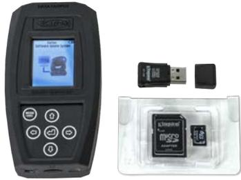
The E-LOADER III™ is a battery powered hand held software uploader device used to update Elation compatible lighting fixtures. Easily upload a software update to an Elation lighting fixture by connecting the uploader to the fixture using the included 3pin DMX cable. All same-type fixtures can be uploaded at once. Elation software updates (not included) are stored on a MICRO SD card (included) and inserted into the uploader.
