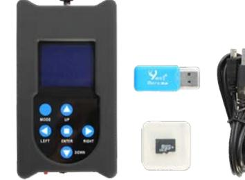
The C loader-II™ is a battery powered hand held software uploader device used to update and test Elation compatible lighting fixtures. Easily upload a software update to an Elation lighting fixture by connecting the uploader to the fixture using a 3pin DMX cable (not included). Elation software updates (not included) are stored on a MICRO SD card (included) and inserted into the uploader. The C-Loader-II™ can also be used as a DMX and RDM Tester.
